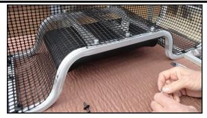
2) Wrap mesh over curved front piece and overlap mesh in middle. Insert remaining push rivets from step 24 into pre drilled holes on curved front piece. Locate 3 Large Head Arrow Connectors from small parts bag-push through mesh into 3 middle pre drilled holes in Carrier Support.
