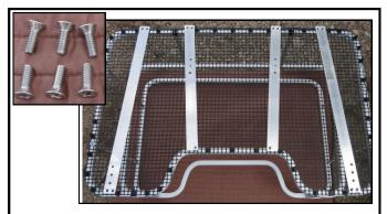
**19)** Locate Flat Head Screws in small parts bag. Position Inner Mounting Straps (P) and Outer Mounting Straps (Q) as shown.
