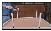
**7)** Take assembled frame bottom and lay flat on table. Tap Lower Front & Rear Vertical Supports (I) onto frame, using hammer and block of wood to prevent bending the ends of tube. Single drill hole on vertical supports must face in.
