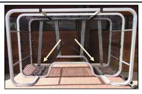
**24)** Insert into all pre drilled holes, including holes in center of vertical supports, up to the holes on front curve. Do not insert into the holes on front curved piece right now.
