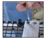
**20)** Attach Mounting Straps using a drop of Liquid Lock Nut onto screw threads. Finger tighten all, then use screwdriver to firmly secure-do not over tighten. \*Can Am machines will have different mounting brackets.
