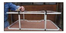
**8)** Take assembled middle of frame, tap onto front & rear vertical supports.
