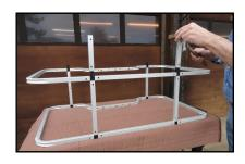
**9)** Tap Top Rear Vertical Supports (J) onto black connectors. Set assembled frame aside.
