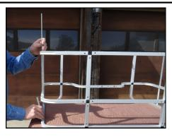
**13)** Take Bottom Vertical Side Supports (K) and Top Vertical Side Supports (L). Line up with holes in frame and insert All Thread Rods (M) through frame and tubing.
