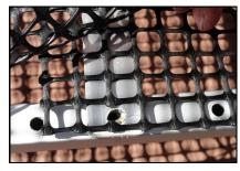
**27)** If needed, cut mesh with razor knife to allow room for bolt. Tighten bolts with 7/16" wrench. Insert remaining push rivets from step 24 into pre drilled holes in curved front piece.
