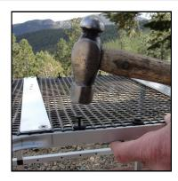
**21)** Tap tops of Push Rivets down with hammer.
