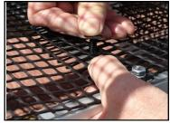
**28)** Locate 3 Large Head Arrow Connectors from small parts bag. Push through mesh into 3 middle pre drilled holes in Carrier Support.
